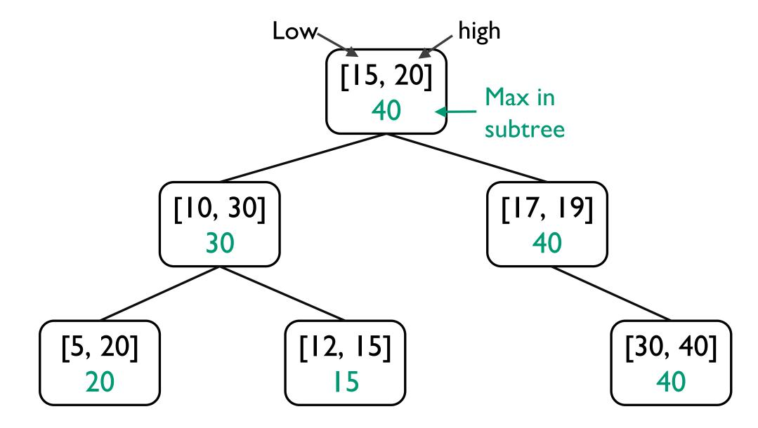
CrossFS uses interval tree to store I/O block ranges for in-flight requests
