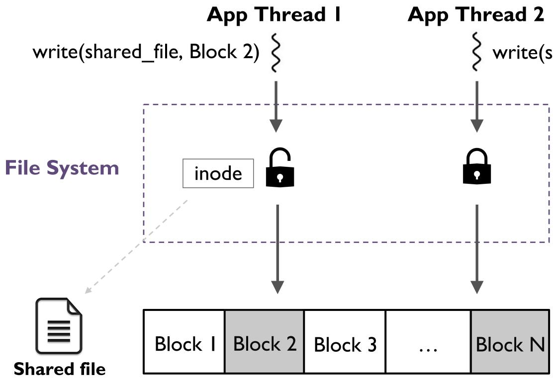
Two threads write to disjoint blocks of a shared file
