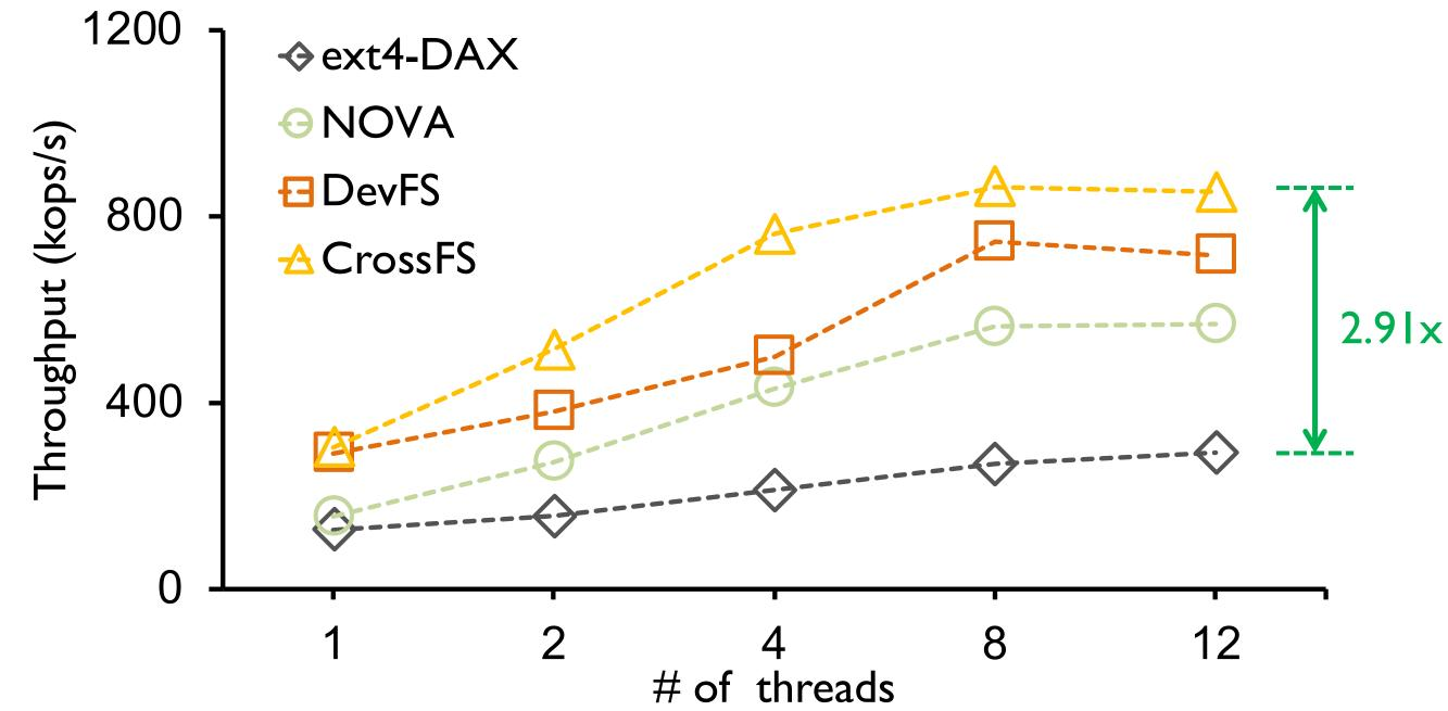
CrossFS writes to NVM buffers first and then asynchronously dispatches request, hence achieves high throughput
